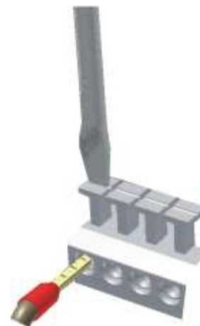
Fig. 8.4 Connecting cables to terminals
